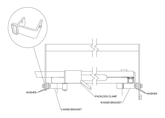
Illustration 2. Linkage guide bracket assembled onto the control valve.
